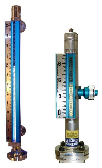
The Jerguson Magnicator is designed to safely determine the level of liquids and liquid interfaces. The operation of the Magnicator is both simple and unique. The patented magnetic circuit provides the best combination for floats and indicators available. The magnets in the float actuate the indicator flags as the level rises or falls. The indicator tracks the float exactly, which in turn provides an accurate level measurement.
