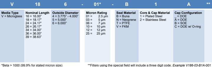
Recommended Operating ConditionsFlow DirectionOutside → InChange Out Differential25 PSIDMaximum Differential150 PSIDMaximum Temperature250° F (Buna)<br/>275° F (Viton)
