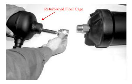
13. Slide float cage / float rod assembly into switch housing. Apply high-temperature thread sealant (Deacon 770P or equal) to 1" NPT Threads.
