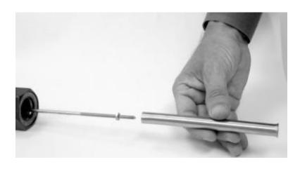
10. Attach (threaded) rod adapter magnet to float rod. Apply Loctite to all male threads prior to installation.
